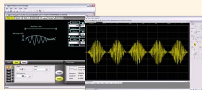
Generate modulated signals internally with scope and function generator
