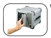
5 Your modular oscilloscope is ready to be plug into an instrument chassis. Using the *Philip* screw driver, screw the L-Mount kit installed on your modular oscilloscope to the instrument chassis (for protective grounding purpose).
