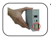
4 To slot in the modular oscilloscope to your chassis, turn your USB oscilloscope model perpendicularly and ensure that the 55-pin back pane connector is at the bottom side of the modular oscilloscope.
