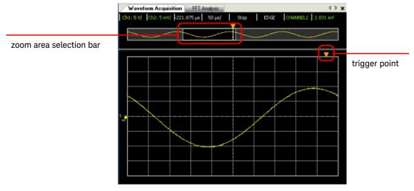
Figure 2-22 Panning a waveform
