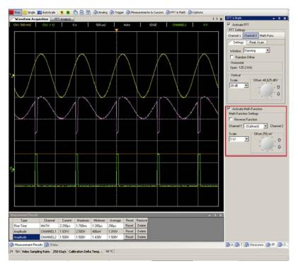
Figure 2-15 Acquired waveform using Subtract function
