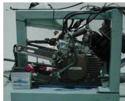
Figure 2. Motorcycle engine mounted for testing
