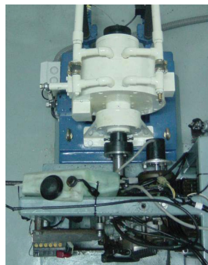
Figure 3. Top view of dynamometer (top) and engine (lower half)
