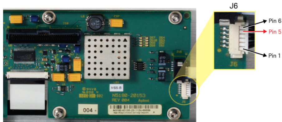
Figure 2-2 A6A1 Front Panel Interface J6 Pinout
