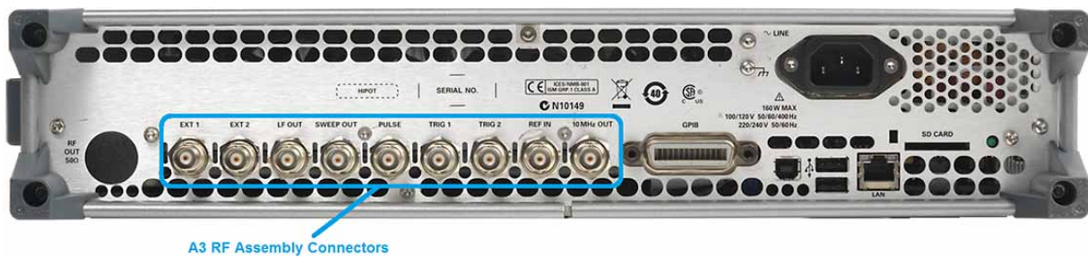
Figure 6-5 N5171B and N5181B Rear Panel BNC Connectors
