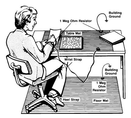
Figure 4. Static-safe Work Station
