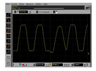
STEP 6: View the jittered pulse on an Agilent 54845A Infiniium oscilloscope.
