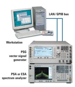
Setup for utilizing Signal Studio software for pulse building to apply pre-distortion to calculated waveforms for improved image rejection and RF flatness.
