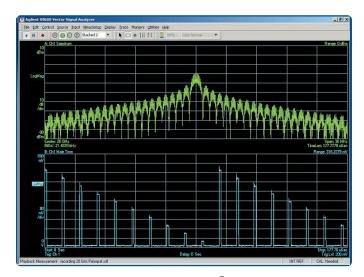
Custom pulse waveform created with MATLAB  $^{\circledR}$  and generated with the E8267C PSG
