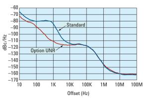
Standard and Option UNR phase noise at 10 GHz from 10 Hz to 100 MHz (all models)
