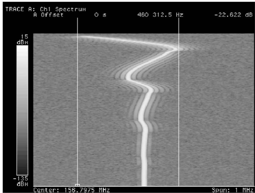
Figure 29. Agilent 89441A spectrogram display for PLL settling time
