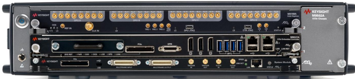
Figure 2. One M9709A digitizer and an M9537A high performance embedded controller installed in the M9502A 2-slot chassis, forming a 32-ch 8-bit standalone acquisition system.
