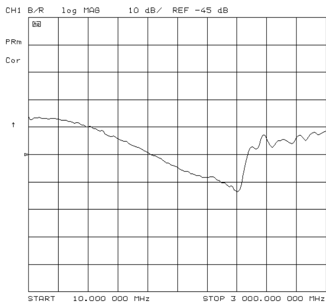
Figure 2-35 Example Mixer LO to RF Isolation Measurement
