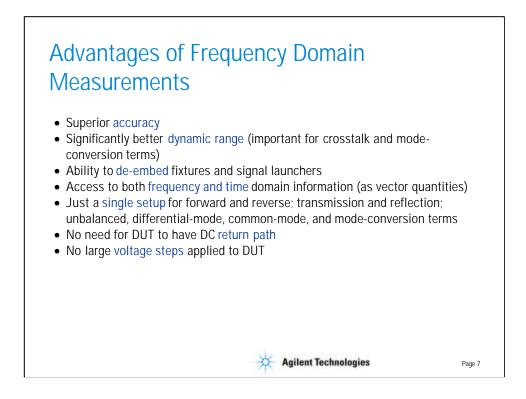
By contrast, a VNA can provide excellent accuracy because the sources of measurement error are characterized during calibration, and a vector error correction is applied to the measured data.
