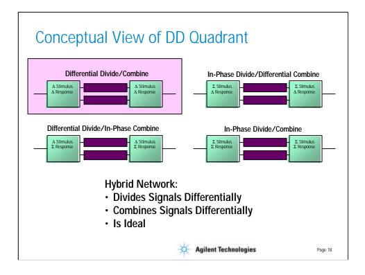
The balanced ports can be converted to single-ended ports. An ideal balun will do this, but the performance will be isolated to the differential mode. The s-parameters of the resulting 2-port single-ended network are the s-parameters in the DD quadrant of the mixed-mode s-matrix.
