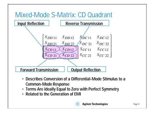
The parameters in the lower left corner describe the common-mode response of a device to a differential stimulus. As with the other modes, there are reflection parameters on each port, and transmission parameters in each direction.
