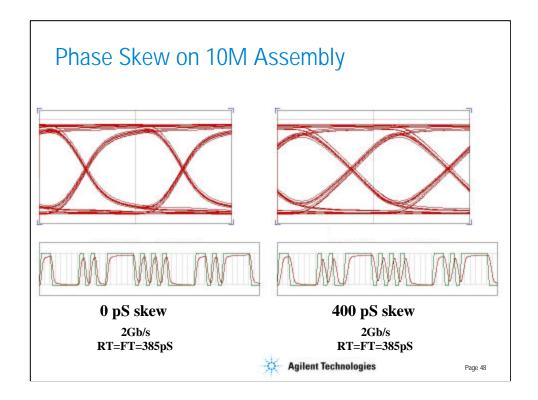
Of course the skew also has an effect on the eye diagram. On the left is the 10 M length of patch cord we have been examining. On the right is the same device with same driving function, but a skew of 400 pS has been introduced. As expected, the resulting eye has begun to collapse.
