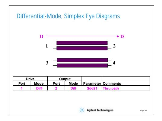
A Fibre Channel cable has two balanced pairs, one for sending data in each direction. The frequency domain measurements described here will fully describe the DUT provided the proper analysis is performed. So far we have concentrated on a single pair operating in one mode at a time. The next few slides will concentrate specifically on a single pair operating in differential mode.
