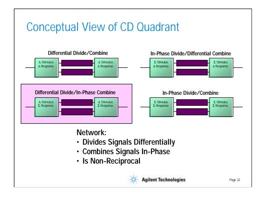
Once again we can convert the balanced port to a single-ended port to understand this mode more conceptually. In this case our network will have to divide the signal differentially as it propagates towards to DUT, and combine signals in-phase as they propagate away from the DUT. Therefore, our network will need to be non-reciprocal in addition to having perfect return loss, insertion loss, balance, and isolation.
