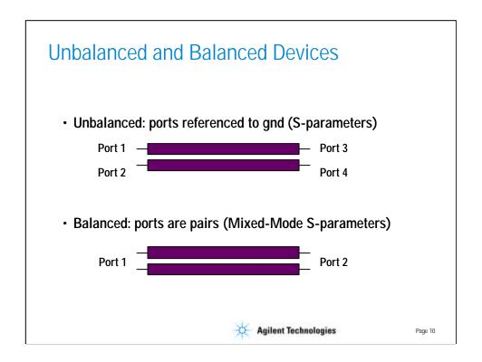
A multi-terminal device can be viewed in different ways, depending on how it is meant to be operated. For a device that is designed to be a single-ended four-port, its conventional four-port s-parameters can be measured and displayed.
