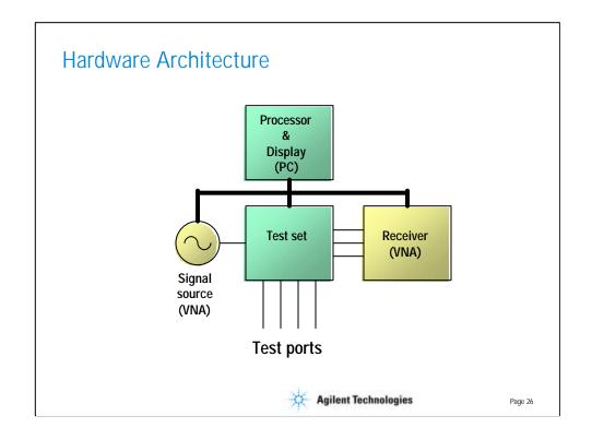
The system that measures balanced devices and display mixed-mode sparameters, uses a combination of hardware and software from Agilent. A 6 GHz system is available using the 8753 VNA and E8357A PNA, as is a 20 GHz system using the 8720.
