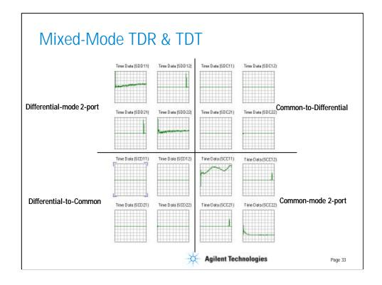
By transforming the frequency-domain data into the time-domain using an FFT algorithm, it is possible to examine the step and impulse responses of the DUT. This can be done on any of the s-parameters, whether they are single-ended parameters, or mixed-mode s-parameters.
