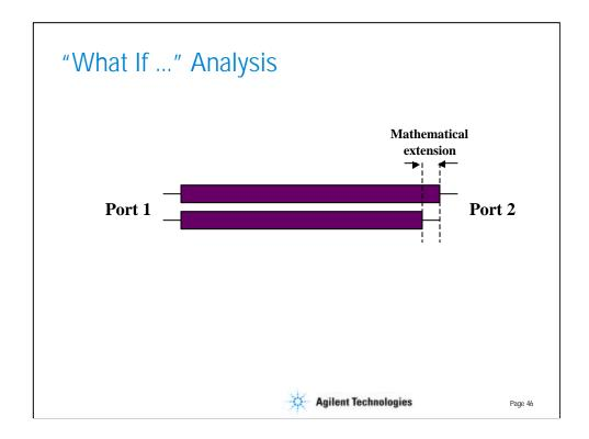
One of the major differences between the TDR and the VNA for characterizing balanced devices is that the TDR provides scalar data, while the VNA provides vector data. Having vector data allows more powerful capabilities, such as better error correction, and features such as deembedding, arbitrary reference impedance definitions, and reference plane rotation (or port extension).
