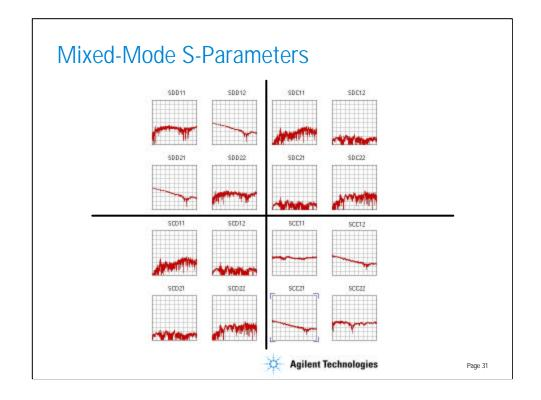
The mixed-mode s-parameters of this cable are shown on this slide. The parameters upper left quadrant describe the behavior in the differential mode. They show a return loss of 20dB at the low end of the band, increasing to about 8dB at the worst point. The loss increases linearly to about 15dB.
