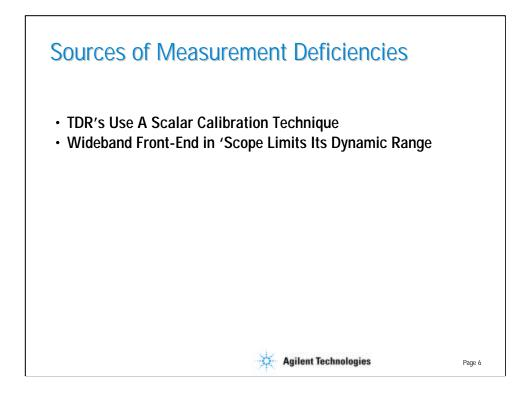
A TDR is a commonly used instrument for testing components such as transmission lines and interconnects. These instruments perform well up to some speed, but eventually their accuracy and dynamic range render them useless.
