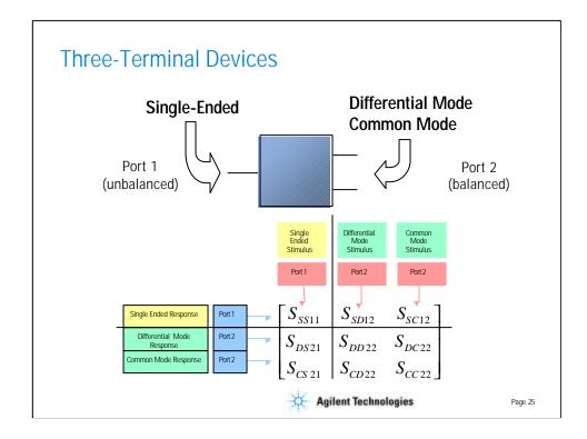
The balanced device that was examined until now has had two balanced ports. A simple extension of the mixed-mode concept can be applied to devices having a combination of balanced and single-ended ports. In this scenario, we need to consider differential and common modes on the balanced ports, and one mode on the single-ended port.
