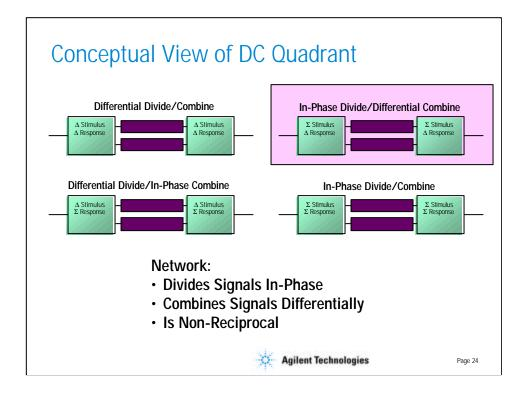
The balanced port can be converted to a single-ended port in this case with a network that divides the signal in-phase as it propagates towards to DUT, and combine signals differentially as they propagate away from the DUT. Once again, our network will need to be non-reciprocal in addition to being ideal.
