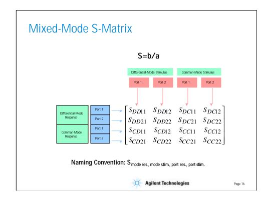
Again we can take a ratio of all of the possible combinations of response over stimulus for the differential and common-mode normalized power waves to calculate the mixed-mode s-parameters.
