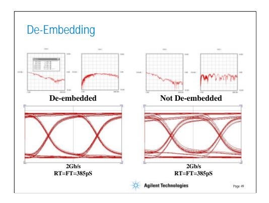
Another of the advantages of vector data is the ability to de-embed. This slide shows a comparison of data with and without de-embedding of the interconnecting lines.
