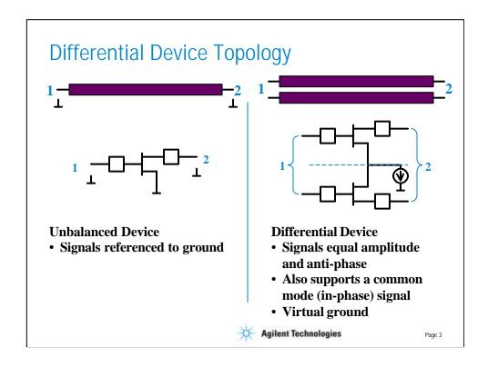
An unbalanced, or single-ended, device has all of its signals referenced to a common ground potential.
