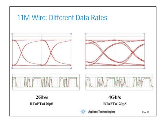
The graphs on the left show the result of using the differential mode sparameter data and generating an eye diagram. The driving function is a data rate of 2 Gb/s with rise and fall times of 120 pS, shown as the green trace below the eye. The resulting output waveform is overlaid in red, shifted in time to be synchronized with the input waveform. This output waveform is then used to generate the eye diagram above.
