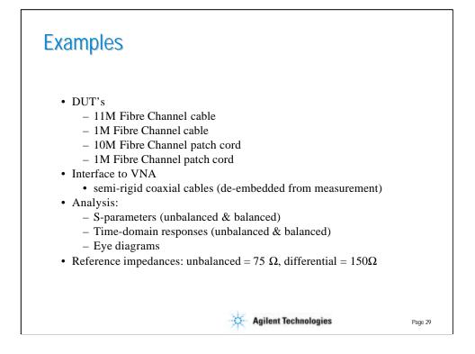
To further understand mixed-mode s-parameters, we will next examine the measured data of several balanced transmissions lines. These devices are all Fibre Channel cables that consist of two balanced pairs, one for sending data in each direction.
