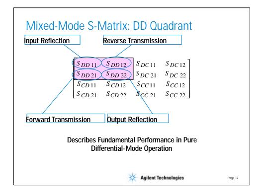
For a device with two balanced ports, the quadrant in the upper left corner of the mixed-mode s-matrix describes the performance with a differential stimulus and differential response. When the performance of the device is isolated to this specific mode, these four parameters describe the input and output reflections, and the forward and reverse transmissions much in the same way a 2-port s-matrix describes the performance of a single-ended device.
