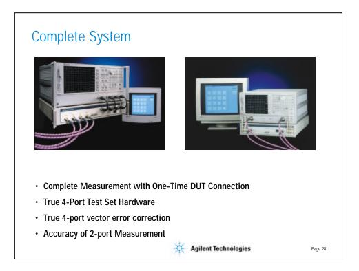
These photos show 6GHz and 20GHz systems that work with the 8753 and 8720 VNA's, respectively. This is a true 4-port measurement system with true 4-port error correction. Designing the systems in this way is essential for obtaining accurate mixed-mode s-parameter data.
