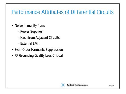
Balanced circuits have been used for many years because of their desirable performance characteristics. They have been mostly used in lower frequency analog circuitry and digital devices, and much less so in RF and microwave applications.
