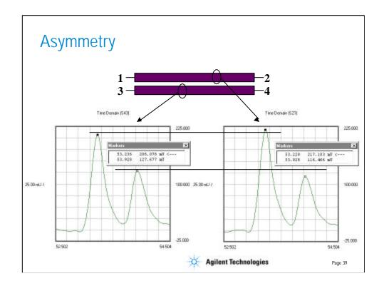
Like any physical device, this one is not perfectly symmetrical. This can be seen by comparing the path from 1-to-2 to that from 3-to-4. The responses look similar, but they are not exactly the same height, and they do not occur at exactly the same times. Therefore, how do we quantify the asymmetry of a balanced device with single-ended measurements?
