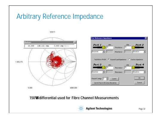
The reference impedance has been set to  $150\Omega$  differential for this device. When a marker is placed at the Sdd11 display at the low end of the band, the impedance readout of the marker confirms that the impedance of the cable is nominally  $150\Omega$ .
