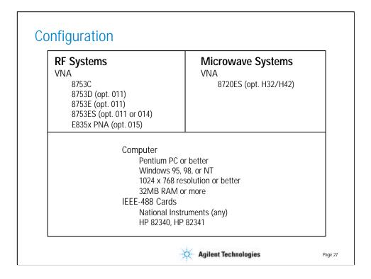
The 6 GHz system that works with the 8753 uses a test set. The 8753 VNA requires either the delete test set option (011) or the configurable test set option (014).
