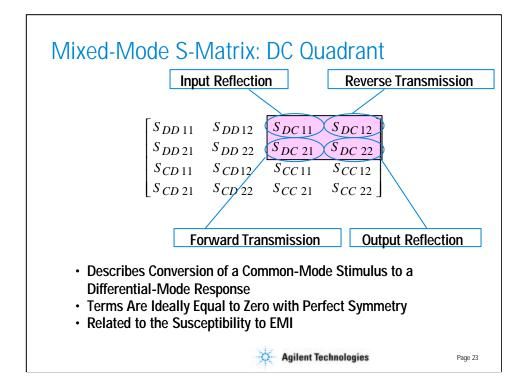
Finally, the parameters in the upper right corner describe the differential response of a device to a common-mode stimulus. Again, there are reflection parameters on each port, and transmission parameters in each direction.
