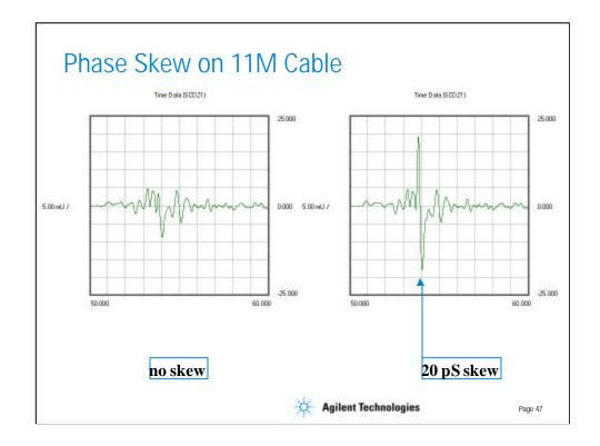
As described earlier, the mode-conversion terms can be used to help determine the cause of asymmetry in a DUT. Even a slight asymmetry can be observed in the time domain. For example, the graph on the left shows the Scd21 parameter of the 11M Fibre Channel cable. If a phase skew of only 20 pS is introduced, the result can be clearly observed, as shown in the graph on the right.
