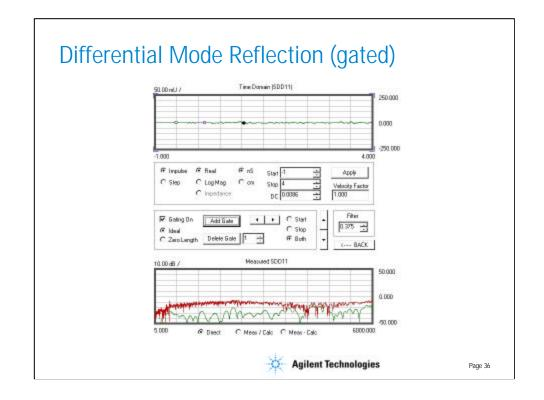
We may want to know what effect the large discontinuity at the input has on the frequency-domain response. The graph at the top of this page shows the time domain response of this device, but with the discontinuity "gated," or mathematically removed.
