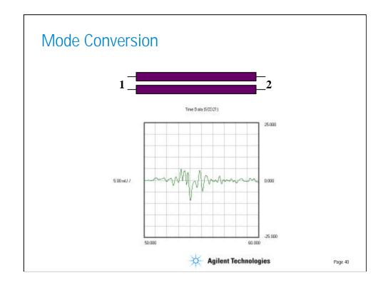
During the review of mixed-mode s-parameters in the frequency domain, we described the mode conversion parameters as being related to the asymmetry. In a perfectly symmetrical device, the mode conversion terms will be equal to zero. We can also examine the mode conversion parameters in the time domain. For example, the Scd21 of this transmission line are shown in this slide.
