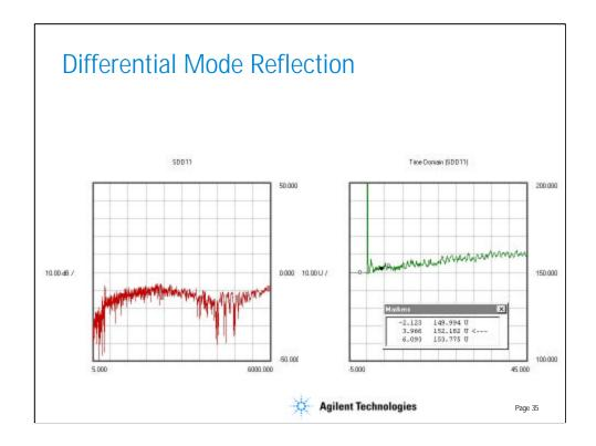
This data shows the differential input reflection performance in the frequency domain and the time domain. The time-domain data is the step response, formatted in ohms on the vertical axis. There is a large discontinuity on the input side as indicated by the spike. This may be responsible for the relatively poor return loss above 1.5GHz.
