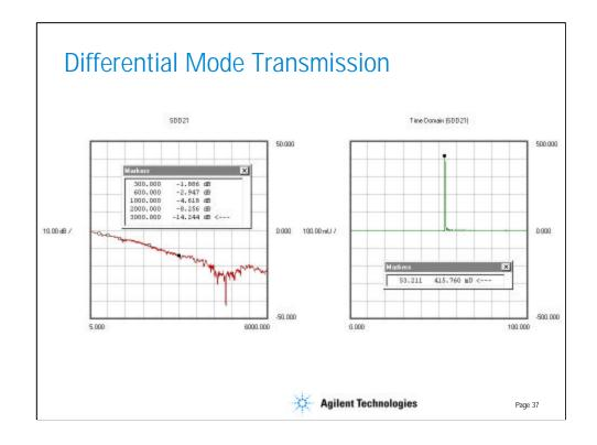
This data shows the differential forward transmission response in the frequency domain and the time domain. The time-domain data is the impulse response. The loss with frequency increases approximately linearly up to about 3 GHz. The group delay is about 53.2 nS.
