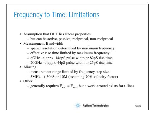
The only assumption that is made about the DUT is that it has linear properties. In other words, its characteristics are independent of the amplitude of the signal. However, the device can be symmetrical or asymmetrical, active or passive, and reciprocal or non-reciprocal.
