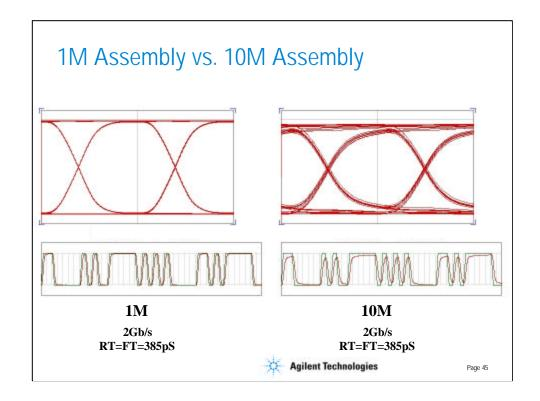
This slide again looks at patch cords, but of two different lengths. One is 1 M long and the other is 10 M long. Clearly the shorter device degrades the signal less than the longer device.
