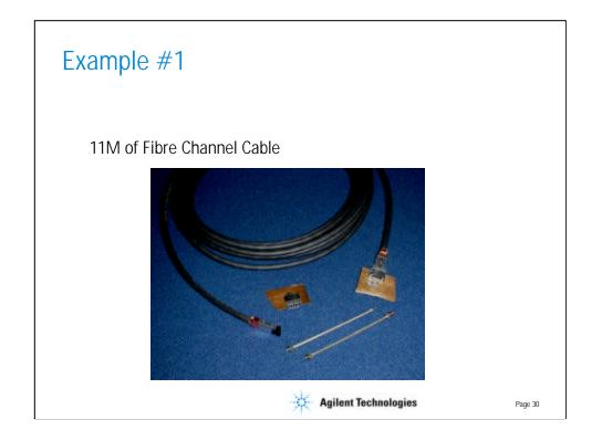
The first device to be considered will be an 11M length of cable. The interface is through SMA connectors attached to short lengths of semi-rigid cable. These semi-rigid cables were characterized to allow them to be de-embedded later.
