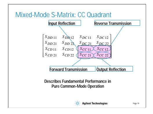
For a device with two balanced ports, the quadrant in the lower right corner of the mixed-mode s-matrix describes the performance with a common-mode stimulus and a common-mode response. When the performance of the device is isolated to this specific mode, these four parameters describe the input and output reflections, and the forward and reverse transmissions.
