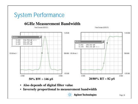
These graphs show the TDT response of the 6GHz system with a through connection (no DUT). This shows the effective impulse width and step rise time. These times are proportional to the maximum measurement frequency, so the pulse width of the 20GHz system is 44pS, and the rise time is 25pS.
