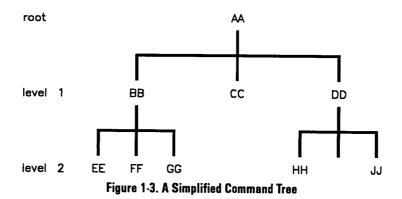
In the command tree shown in Figure 1-3, the command closest to the top is the *root command*, or simply the *root*. Notice that you must follow a particular *path* to reach lower level subcommands. For example, if you wish to access the **GG** command, you must follow the path **AA** to **BB** to **GG**.
