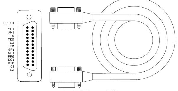
Figure 1-1. HP-IB Connector and Cable
