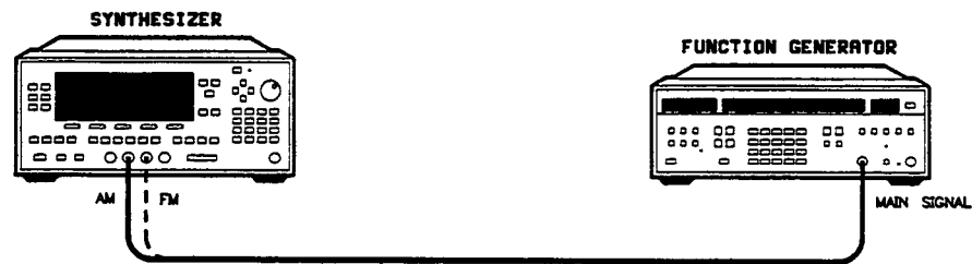
Figure 2.26. Modulation Meter Test Setup
