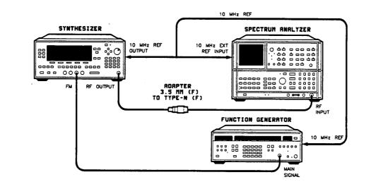
Figure 2-22. FM Accuracy Test Setup
