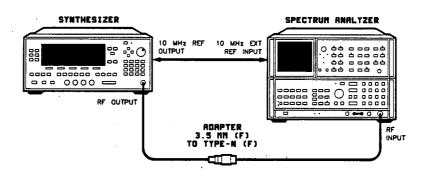
Figure 2-9. Spurious Signals (Harmonic) Test Setup
