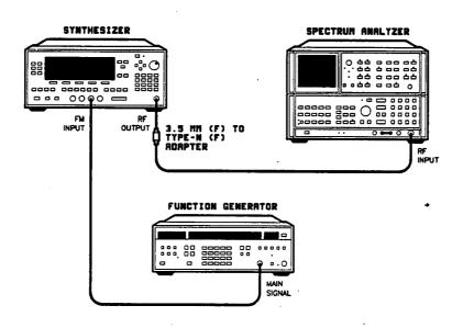
Figure 3-36. FM Gain Adjustment Setup
