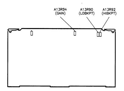
Figure 3-13. YO Gain and Linearity Adjustment Locations
