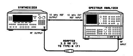
Figure 2-10. Spurious Signals (Non-Harmonic) Test Setup
