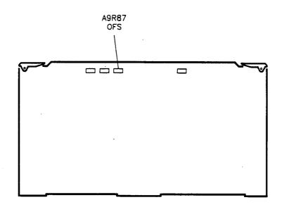
Figure 3-15. Amplifier Detector Offset Adjustment Location
