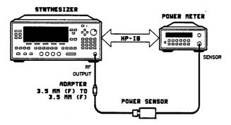
Figure 3-29. Power Flatness Adjustment Setup
