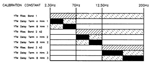
Figure 3-17a. Single-Band Delay and Risetime Compensation
