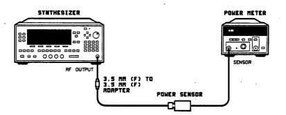
Figure 3-38. Square Wave Symmetry Adjustment Setup
