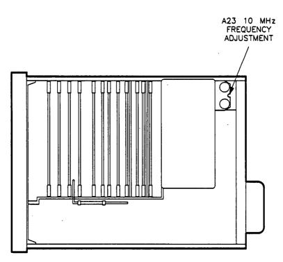
Figure 3-2. 10 MHz Standard Adjustment Location
