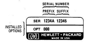
Figure i. Typical Serial Number Label
