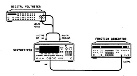
Figure 3-32. AM Delay Adjustment Setup
