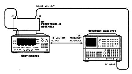
Figure 3-5. Fractional-N Reference and API Spur Adjustment Setup
