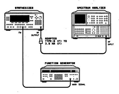
Figure 2-24. Maximum FM Deviation Test Setup
