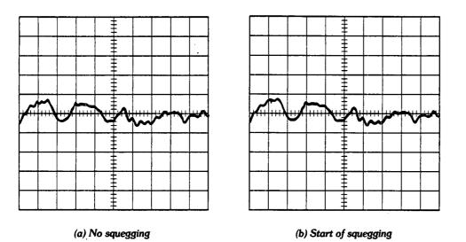
Figure 3-19. Squegg Clamp Band 1 Adjustment
