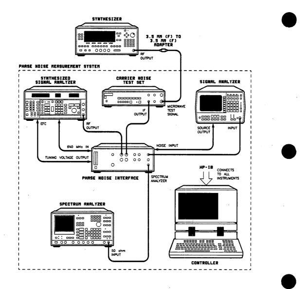
Figure 2-12. Single Sideband Phase Noise Test Setup
