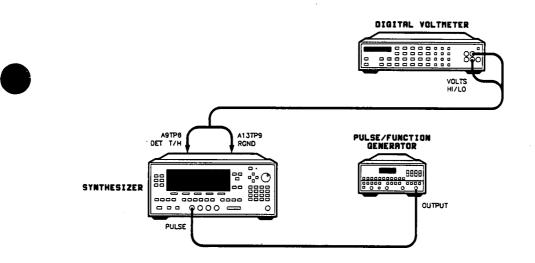
Figure 3-34. Pulse Delay Adjustment Setup
