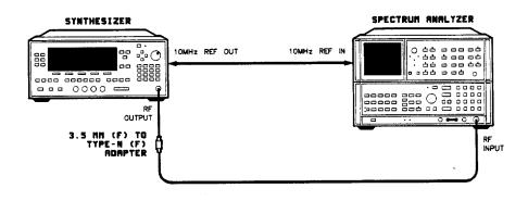
Figure 2-13. Alternate Phase Noise Test Setup
