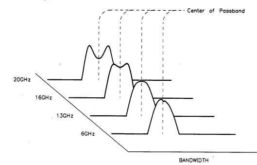
Figure 3-16. SYTM Passband Versus Frequency
