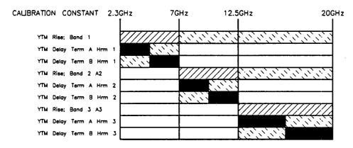
Figure 3-17a. Single-Band Delay and Risetime Compensation
