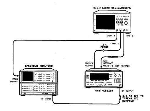
Figure 2-2. Swept Frequency Accuracy Test Setup
