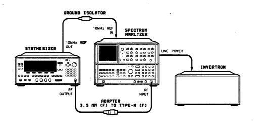
Figure 2-11. Spurious signals (Line-Related) Test Setup
