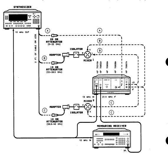
Figure 4-1. Step Attenuator Flatness Setup
