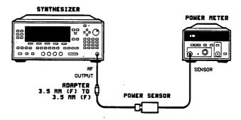
Figure 3-27. ALC Power Accuracy Adjustment Setup
