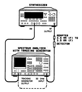
Figure 2-20. AM Bandwidth Test Setup
