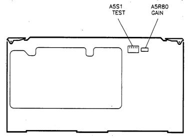
Figure 3-14. Switch and Adjustment Locations
