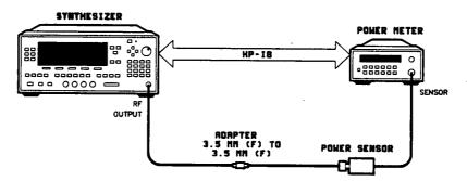
Figure 2-6. Power Flatness Test Setup
