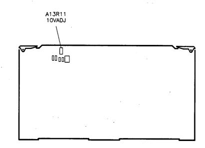
Figure 3-11. YO Driver +10V Reference Adjustment Location
