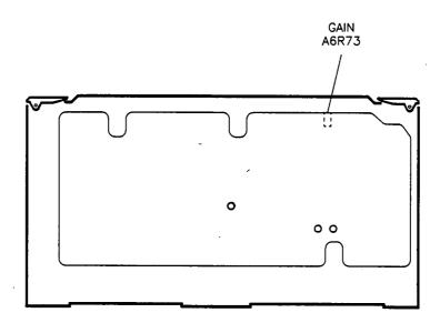
Figure 3-9. IF Gain Adjustment Location
