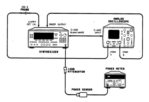
Figure 3-18. SYTM Adjustments Setup
