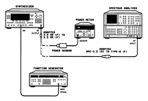
Figure 2-21. AM Dynamic Range Test Setup
