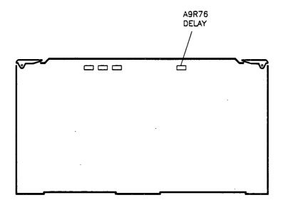
Figure 3-35. Pulse Delay Adjustment Location
