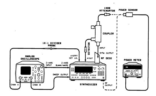
Figure 3-18. SYTM Adjustments Setup
