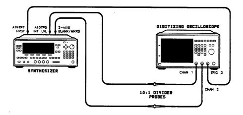
Figure 3-22. Low Power SRD Bias Adjustment Setup
