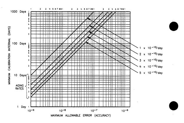
Figure 3-3. Accuracy Versus Adjustment Interval
