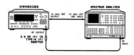
Figure 2-14. Pulse Modulation On/Off Ratio Test Setup
