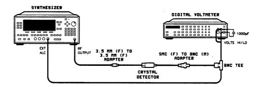
Figure 2-8. External Leveling Test Setup
