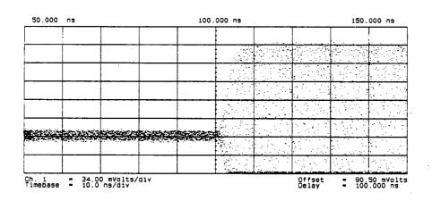
Figure 2-16. Signal Level between RF Power Off and On
