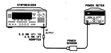
Figure 2-5. Power Accuracy Test Setup
