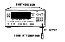
Figure 2-7. Maximum Leveled Power Test Setup
