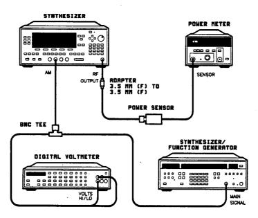
Figure 3-30. AM Accuracy Adjustment Setup
