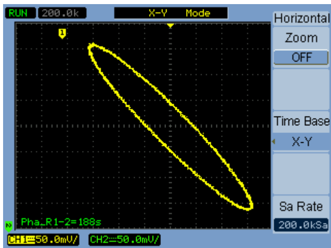
Figure 14 X-Y Display Format Showing Out-of-Phase Waveforms
